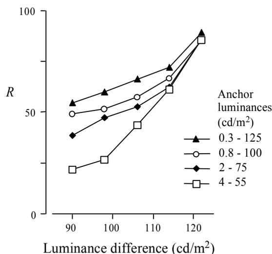
**Figure 2.** Mean rating  $R$  of darkness as a function of absolute luminance difference between stimulus and background for each pair of anchor luminances.
